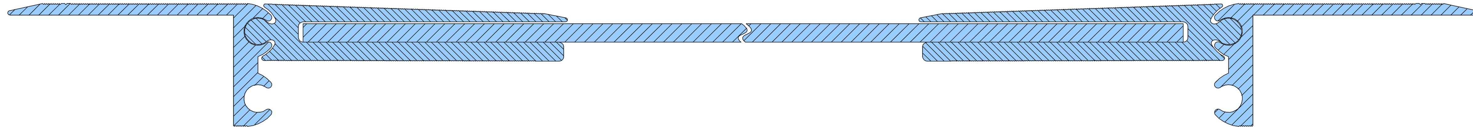
*The profile is made for a specific width of the expansion joint "A" (mm) from 300 to 1000 mm*
