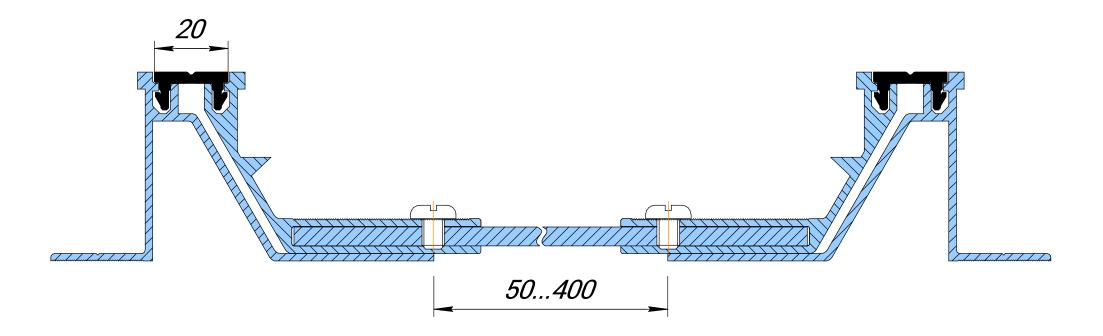
The profile is made for a specific width of the expansion joint "A" (mm) from 50 to 400 mm
