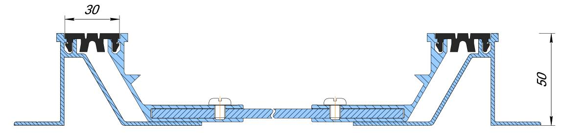
The profile is made for a specific width of the expansion joint "A" (mm) from 50 to 400 mm
