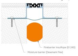
The profile can be made to order for the required height from 50 to 200 mm. In this case, it is completed with an assembled frame consisting of an aluminum guide and a steel angle.
