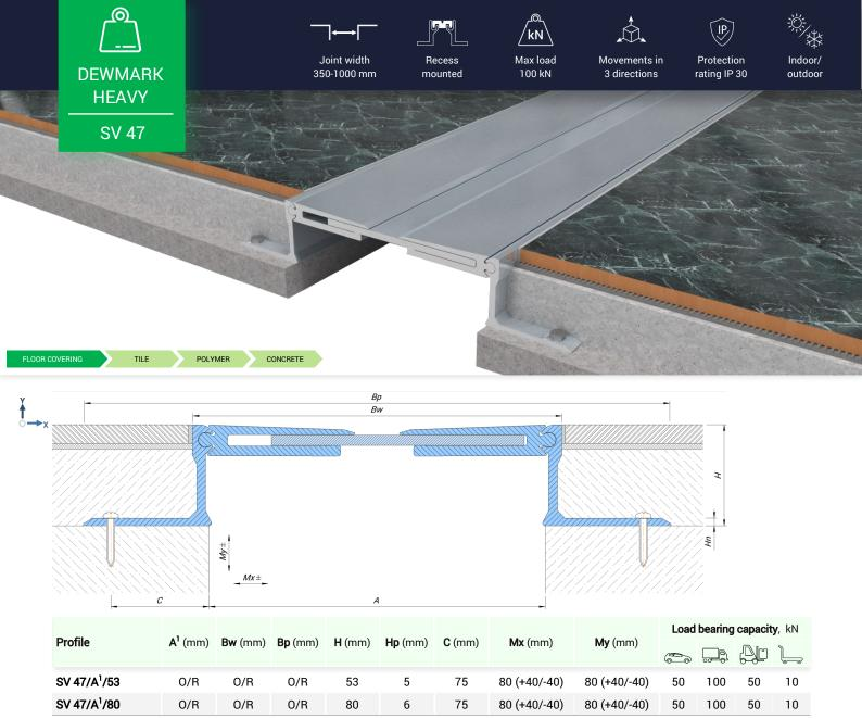
!<sup>1</sup> The profile is selected on a specific width of the expansion joint "A" from 350 to 1000 mm.
